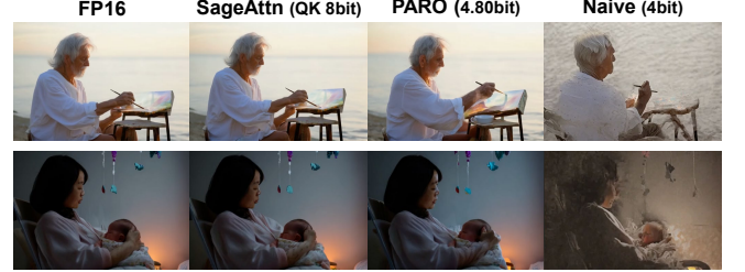
Fig. 7. Comparison of generated videos for different quantization methods. The PARO quantization method could generate videos without visual difference with FP16 generated videos with an averaged of 4.80bit.
