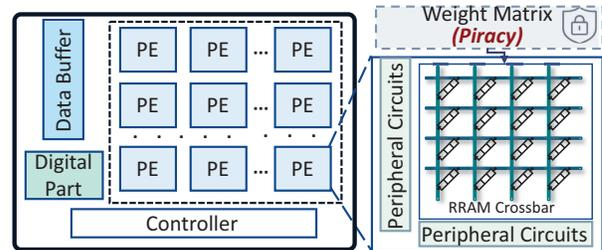
Fig. 1. Basic structure of an RRAM computing system
