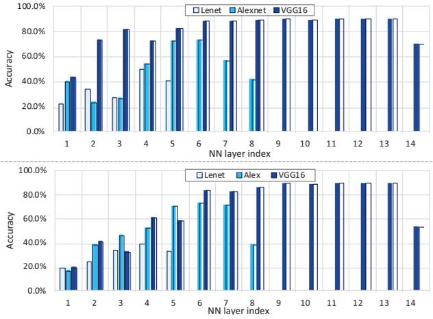
Fig. 4. Classification accuracy of extracted NN models with obfuscating only one single layer for *Up*: analog RRAM; *Down*: digital RRAM. Lower accuracy means the layer has more significant impact on the NN model
