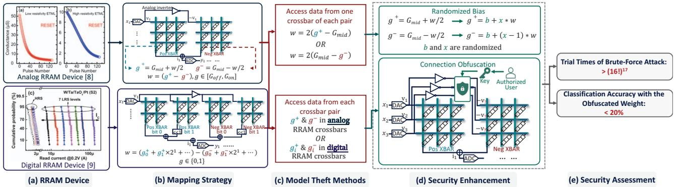
Fig. 2. Overview of the proposed methods: (a) the characteristics of analog RRAM and digital RRAM; (b) the different mapping methods for analog RRAM and digital RRAM; (c) two model theft methods; (d) the security enhancement to counter the theft methods; (e) the security assessment after applying the security enhancement.
