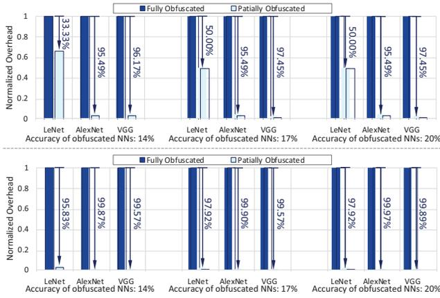
Fig. 6. Hardware area overhead reduced by obfuscating only partial NN layers and weight bits under three obfuscation object thresholds compared with fully obfuscating all layers and all bits. *Up*: analog RRAM; *Down*: digital RRAM
