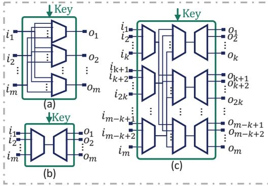
Fig. 3. Different implementation of the obfuscation module: (a) each time  $m$  inputs and  $m$  output are connected; (b) each time only 1 input and 1 output are connected; (c) combines (a) and (b) so that each time  $x$  inputs and  $x$  outputs are connected.
