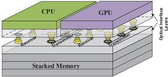
Fig. 4. Diagram of OAM-based wireless chip-to-chip optical interconnect
