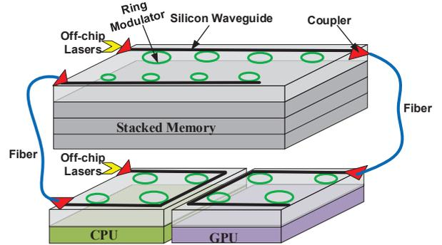
Fig. 2. Diagram of fiber-based traditional chip-to-chip optical interconnect
