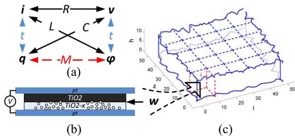
Figure 1. (a) Memristor is the fourth basic circuit element. (b) The ideal TiO<sub>2</sub> memristor model. (c) The geometric variation model.
