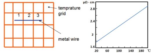
(a) metal wire in thermal grids (b) temperature impact on resistivity
