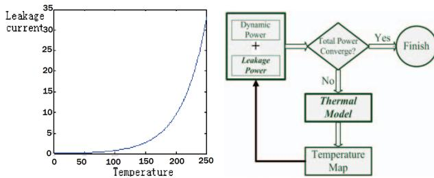
(a) leakage increase with temperature (b) iterative estimation process
