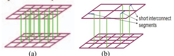
Figure 2. 3D uniform Grid(a) and non-uniform(b)
