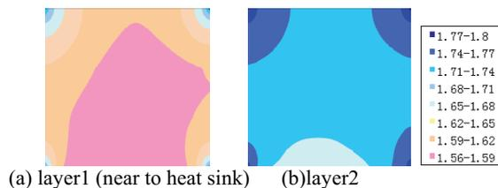
Figure 1. Voltage distribution in different layers\*
