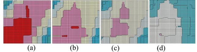
Figure 8: IR drop under different TSV-insertion method: (a) IR drop without insertion of P/G TSVs ;(b) IR drop with insertion of P/G TSVs by *Uniform\_Grid* ;(c)IR drop analysis after inserting TSV by *Max\_Diff* approach ;(d) IR drop with insertion of P/G TSVs by our method (the parameters in Algorithm 1 as  $\varepsilon_1 = 1 \times 10^{-6}$ ,  $\varepsilon_2 = 1 \times 10^{-7}$ )
