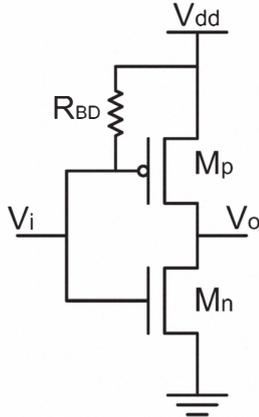
Fig. 1. Breakdown resistance in pMOS device in the inverter
