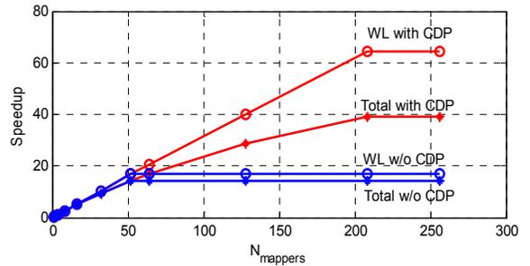
Figure 13. The speedup of different mapper numbers
