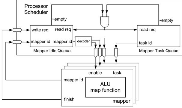
Figure 5. The internal structure of mapper scheduler
