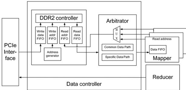
Figure 10. The internal structure of data controller
