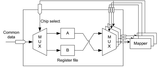
Figure 6. The internal structure of common data path
