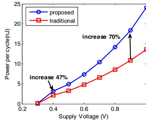
**Figure 14. Power analysis of the two buffers.**
