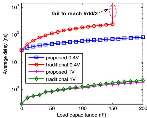
**Figure 7. Buffer sensitivity to load capacitance.**
