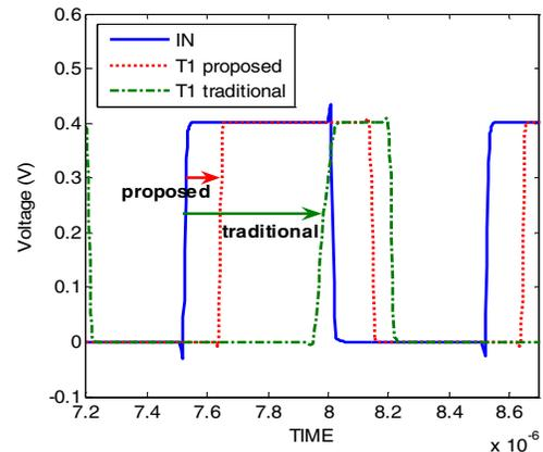
Figure 12. Clock waveform comparison between two buffers.
