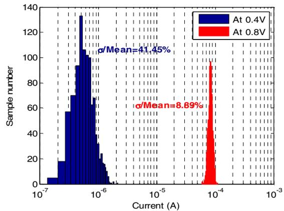
Figure 3. Current variation with different gate voltages.
