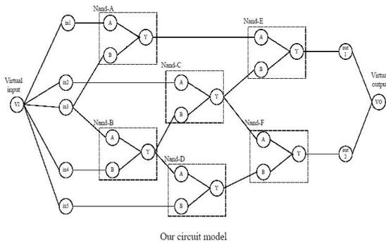
**Figure 2.** Signal-path level circuit model (C17).
