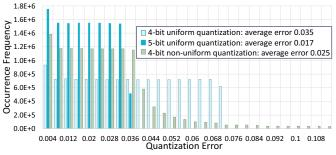
Fig. 3. Quantization error distributions under different quantization methods (i.e., 4-bit uniform quantization, 5-bit uniform quantization, and 4-bit nonuniform quantization)
