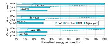
Fig. 5. The normalized energy consumption of each part (A6W4(6): existing work with traditional quantization method; Opt.1: optimized by nonuniform quantization scheme; Opt.1+2: optimized by non-uniform quantization scheme and energy-aware weight regularization)
