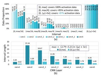
Fig. 2. (a) The percentage of activation data in different ranges w.r.t. different CNN layers in a well-trained VGG-8 model. (b) The quantization range sizes in different layers.
