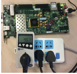
Figure 10: Testing platform. We use Xilinx Zynq ZC706 for on-board testing. A power meter is used for power analysis.
