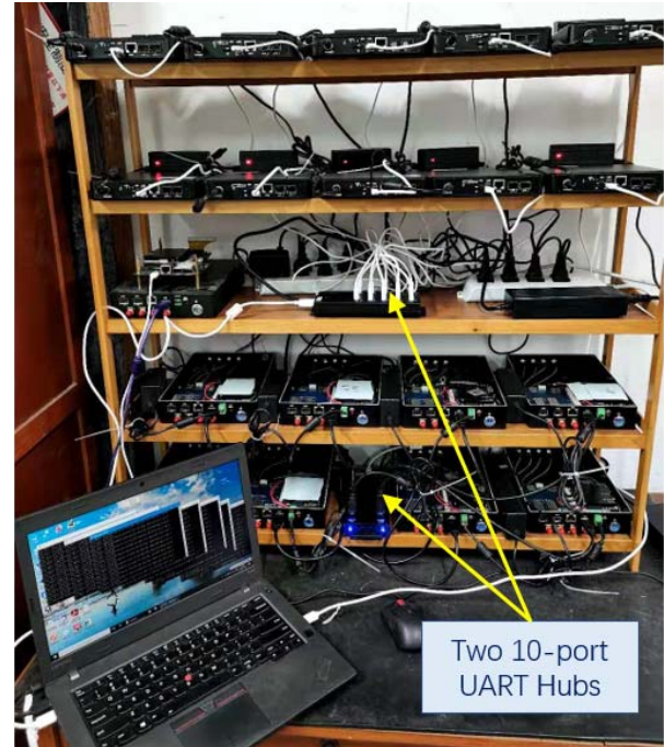
Fig. 8. Fault injection platform with 20 XC7Z045 boards.
