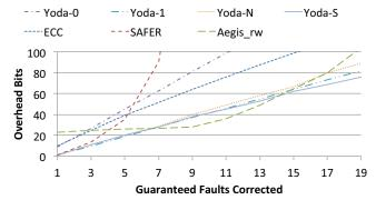
Fig. 2: Overhead bits to guarantee a particular fault-tolerance.
