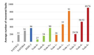
Fig. 3: Faults corrected before failure in a 4KB page. The number of auxiliary bits per block is shown above its bar. For Yoda, the overhead is shown for regular and small Yoda, respectively.
