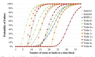
Fig. 4: Probability of failure with various stuck-at faults per data block under protection of different recovery schemes.
