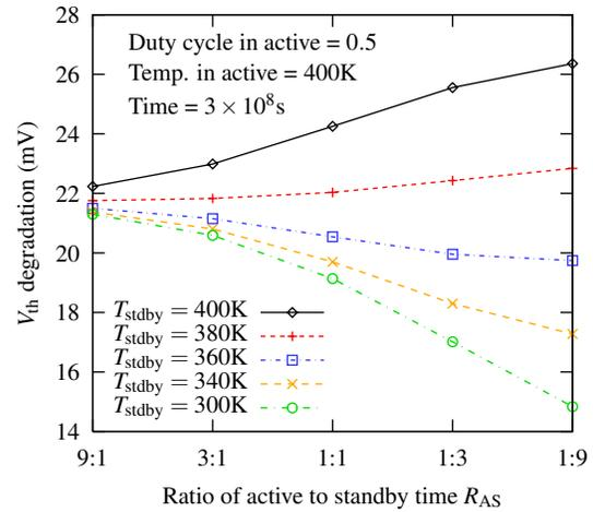
**Figure 6. Impact of  $R_{AS}$  on  $V_{th}$  degradation**
